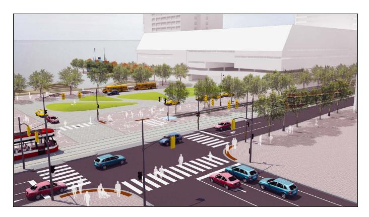
**Figure 5** – Artist's depiction of typical Queens Quay East street cross-section with at-grade streetcar extension. Proposed alternate tunnel portal and Yonge Street Slip fill-in also shown.
